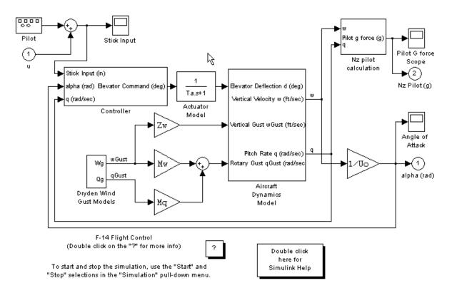
The model simulates the pilot's stick input with a square wave having a frequency of 0.5 radians per second and an amplitude of  $\pm$  1. The system outputs are the aircraft angle of attack and the G forces experienced by the pilot. The input and output signals are visually monitored by Scope blocks.
