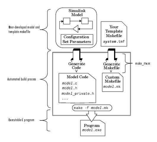
A high-level M-file command controls the Real-Time Workshop build process. By default, Real-Time Workshop issues the command make\_rtw with appropriate options for most targets. You can customize this command by editing the contents of the **Make command** field in the **Build process** section of the **Real-Time Workshop** pane of the Configuration Parameters dialog box.
