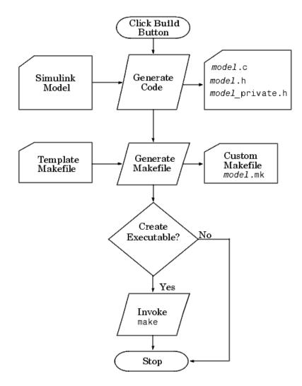
During the final stage of processing, Real-Time Workshop invokes the generated makefile, *model*.mk, which in turn compiles and links the generated code. On PC platforms, a batch file is created to invoke the generated makefile. The batch file sets up the proper environment for invoking the make utility and related compiler tools. To avoid unnecessary recompilation of C files, the make utility performs date checking on the dependencies between the object
